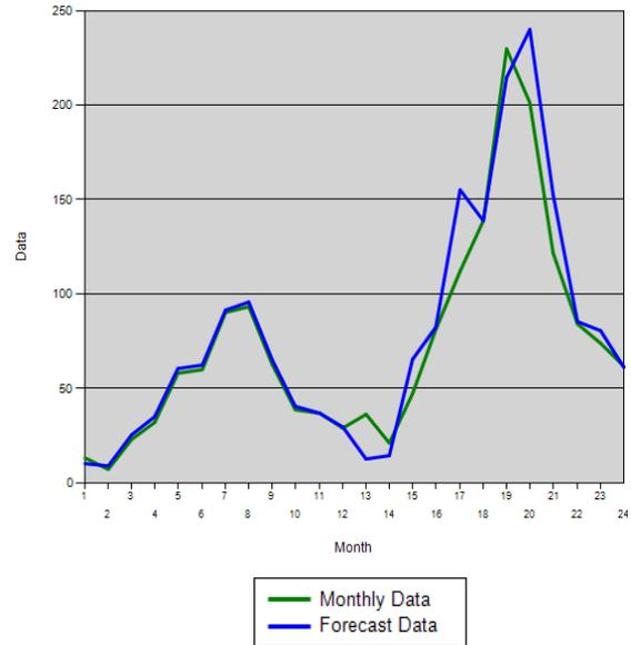
**Figure 4.** Winter's method forecasting ( $\alpha = 0.6, \beta = 0.1, \gamma = 0.9$ )
