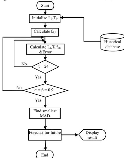
Figure 1. Flow chart of Holt's method
